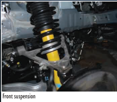
Suspension well shielded from overspray of wheel arch treatment then lacquered
