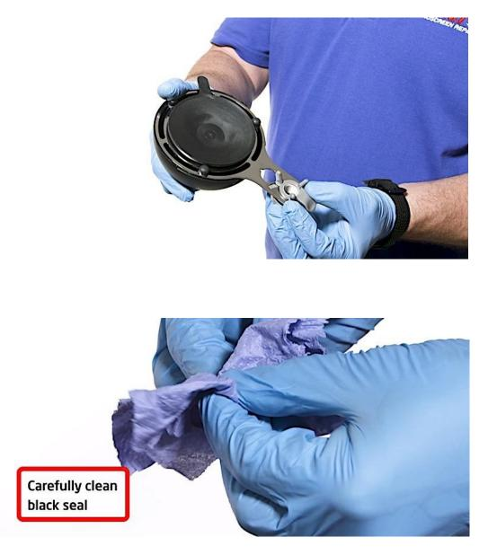
To clean the syringe assembly, remove the needle and plunger and carefully clean the black seal on the plunger.
