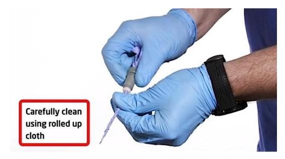
It is especially important to clean the injector seal very carefully, completely wiping away any excess resin. This will prolong the life of the injector.
