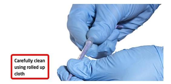
The inside of the syringe can be dried using a rolled-up piece of dry cloth. Any residual resin should also be removed from the needle.
