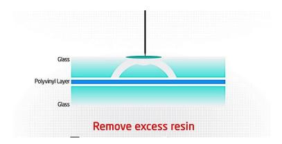
Press down firmly whilst moving the blade rapidly back and forth and in different directions.
