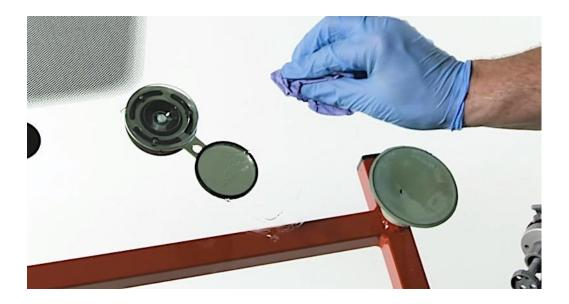
Take a small pre-cut square of mylar film and the bottle of pit fill resin.
