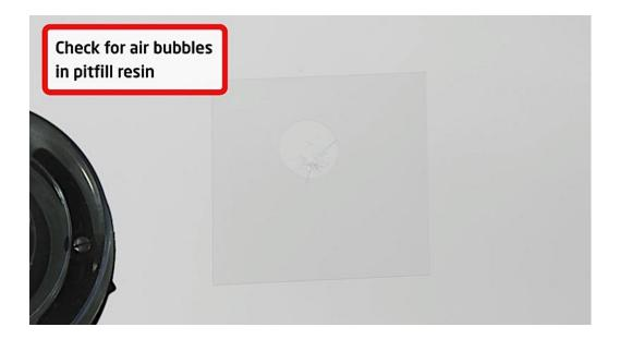
Take the UV lamp from the case and place over the area to be cured, pressing down firmly, and using a "rocking" action to expel the air from the suckers.
