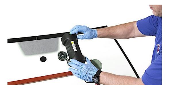
After curing, gently remove the UV lamp by lifting the tab of each sucker.
