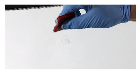
Once the excess resin is removed, use a cloth to take a small dab of pit fill polish from the jar and rub this over the impact crater around the glass. After about a minute the transparency of the screen should be greatly improved.
