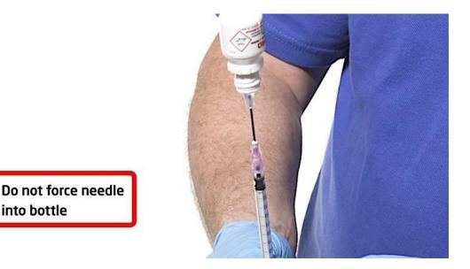
A typical repair will use 0.2ml of resin. To load the resin, first carefully draw the plunger back to 0.4ml, then push back to 0.2ml. This ensures there is no air present in the syringe and needle.
