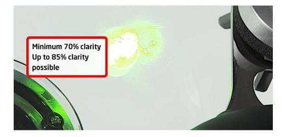
If you are repairing a 'star' break, bring your eyeline close to the windscreen surface and inspect along each individual crack of the star. When looking from this angle, each line of damage should have disappeared.
