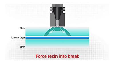
Creating too much pressure will cause the injector seal to blow, and the resin to leak. You can avoid this by monitoring the injector seal with the attached mirror.
