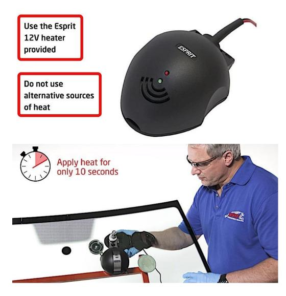
Test the temperature of the glass using the back of your forefinger and repeat the 10 second warming process for as many times as necessary to warm the glass to slightly above skin temperature.
