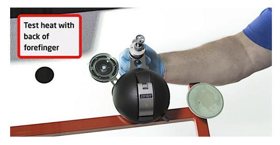
Take care not to overheat the glass as too much heat will close-up the cracks and fissures.
