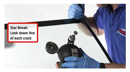
Once the resin has been applied and you are satisfied that the damage is cleared you are ready to cure the **resin with the UV lamp**.
