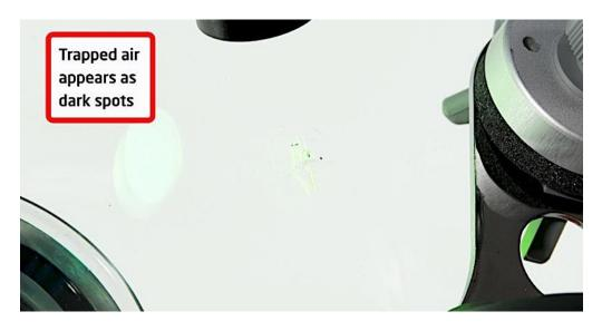
A full repair will usually require two or more cycles. Before reapplying a second time, you need to gently warm the screen to expand cracks and fissures and aid the ingress of resin.
