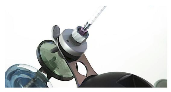
Take the male plunger and gently screw this into the female injector. As the plunger is screwed down, it will force the resin into the break.
