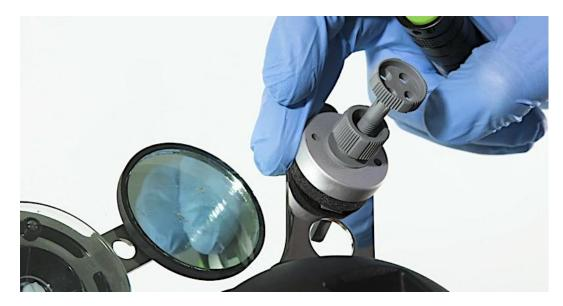
Great care should be taken in trying to identify any remaining sigs of damage or trapped air prior to curing. Use the LED torch to assist with the visual inspection.
