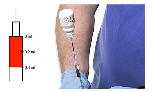
Gently place the needle all the way into the open end of the injector barrel and inject the resin so that it falls onto the damage.
