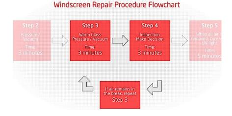
The final inspection of the break is the most important stage of the repair.
