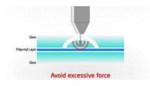
• Do not apply excessive force or push the drill too deeply into the glass during the cleaning process, as this could damage the polyvinyl layer that lies between the inner and outer sheets of glass.
