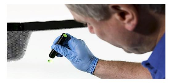
The Esprit system can be used on chips up to 40mm. But to comply with the British Standard, the size of the damage in certain areas is important. In the 'A-zone', which is immediately in front of the driver, only damage up to 10mm can be repaired. If the damage is in the 'C-zone' – in front of the passenger seat – then chips up to 25mm can be repaired safely.
