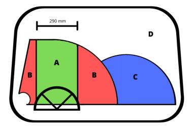
Identify the correct zone on the windscreen where the break is located. Use the clear overlay provided within the kit to ensure that the size of the damage is within the limit for that zone.
