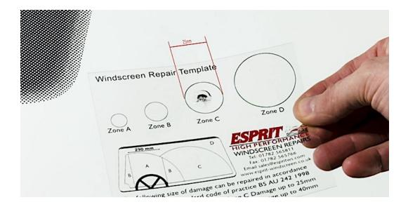
Next, you need to identify the precise point where the stone has struck the glass. This is known as the impact crater. For a successful repair, the impact crater should be no larger than 5mm in diameter. Using the inspection tool, scratch into the impact crater. If you hear a grinding or scratchy sound, this means that the impact crater is blocked with glass debris, dirt or moisture.
